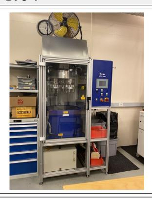
Finishing machine for processing parts, cutting tools and tooling
